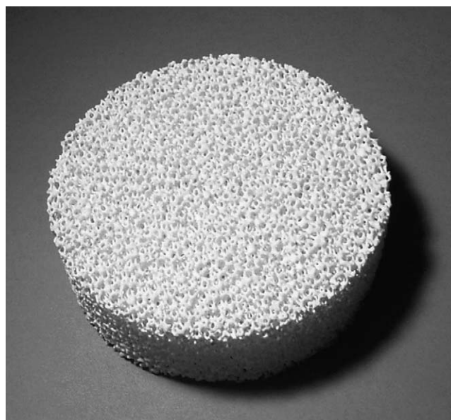
Fig. 1. Photograph of an open cell ceramic foam piece.
